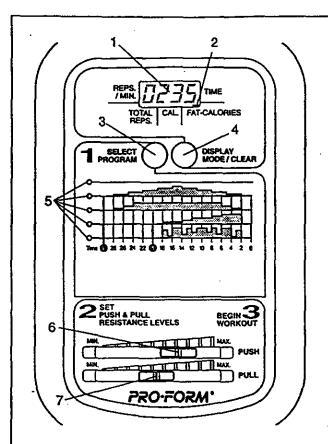
1. LCD display-Displays the six monitor modes.
